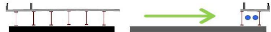
Phase 3 – Bridge Closed to Traffic, Existing Bridge Superstructure Removed, and New Bridge Superstructure Slid to Final Location
