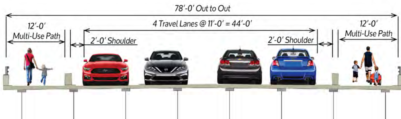
Fig. 8 - Proposed Bridge Typical Section
